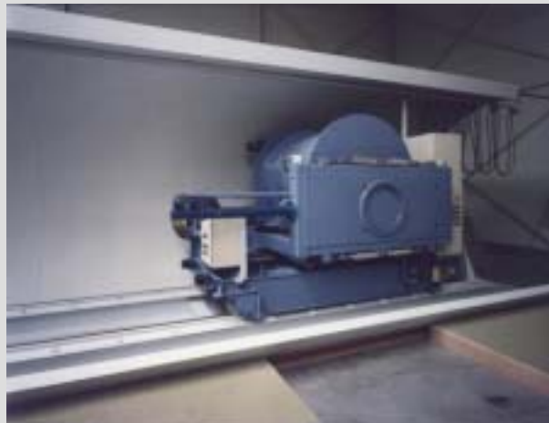
Figure 3.30 The handling device for the overpacks of vitrified waste being demonstrated in the HADES–PRACLAY hall.
