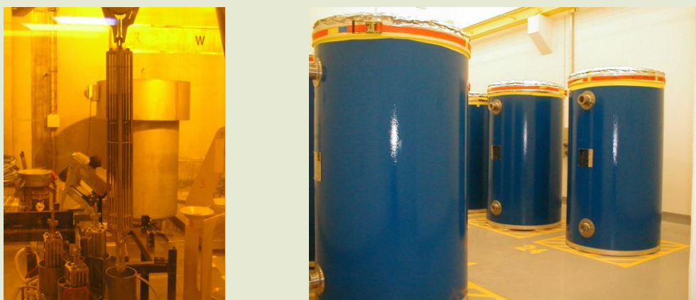
Figure 8 – Unloading of irradiated fuel from Ghent University's Thétis research reactor at Belgoprocess (source: Belgoprocess) and storage of irradiated fuel from SCK•CEN's BR3 research reactor in Castor containers on the BP1 site of ONDRAF/NIRAS operated by Belgoprocess (source: Belgoprocess / ONDRAF/NIRAS).
