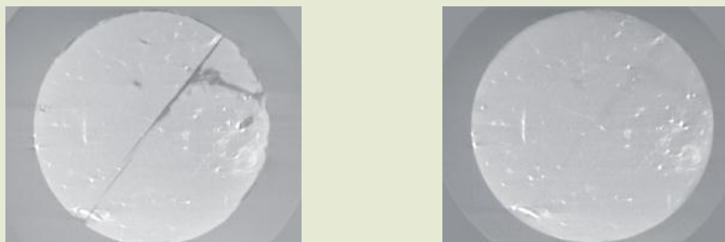
Illustration of the self-sealing capacity of Boom Clay. Left: clay sample in which a fracture has been induced; right: the same sample 4 hours after hydraulic saturation: the fracture has been sealed.
