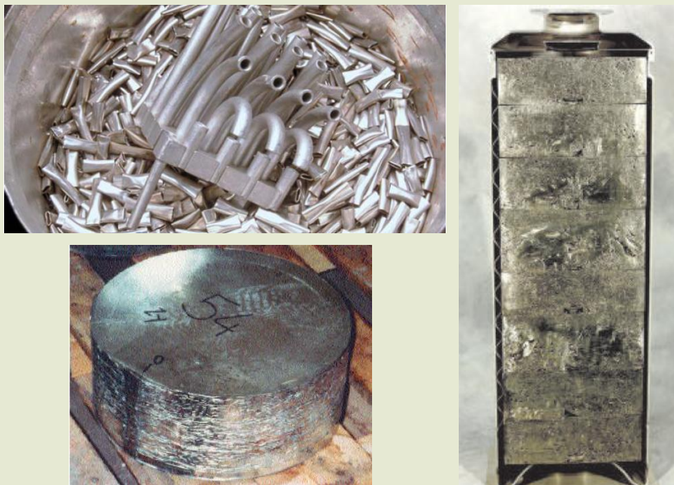
Figure 14 – Metal waste from the reprocessing of irradiated nuclear fuel (upper left) and the same waste compacted into slabs (lower left) then put into stainless steel containers (right) (source: AREVA NC).
