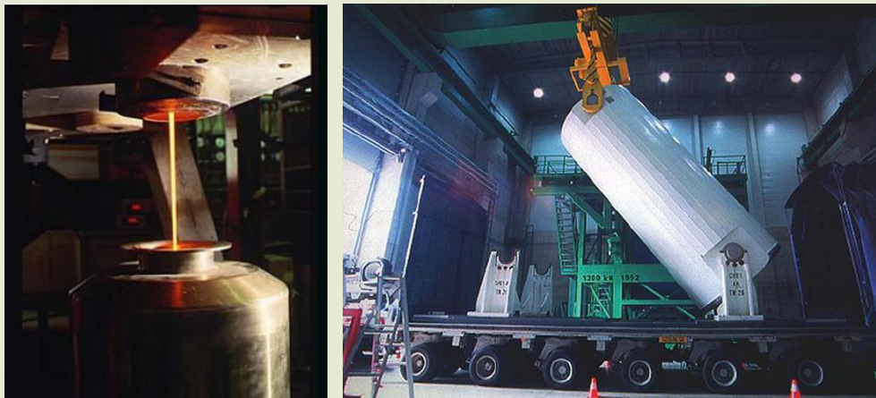
Figure 9 – Filling of a container of vitrified waste from reprocessing (source: AREVA NC) and transfer of a shielded transport container containing 28 containers of vitrified waste (source: Belgoprocess).
